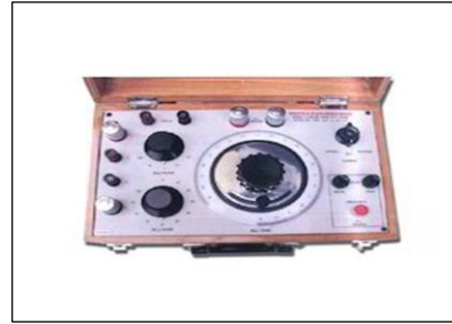
fig. Kelvin Bridge
