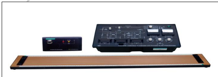
Calibration of Voltmeter using Potentiometer
